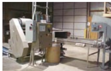
Kard's Allegheny 36-1000C, 100 Hp. shredder.
